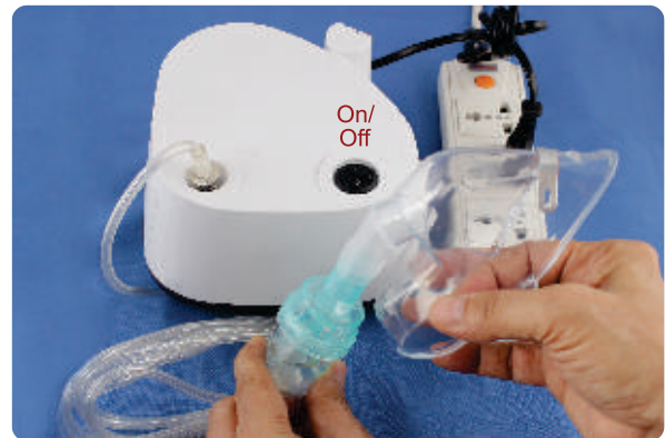
Step 3. Close the chamber, connect mask & start the machine
