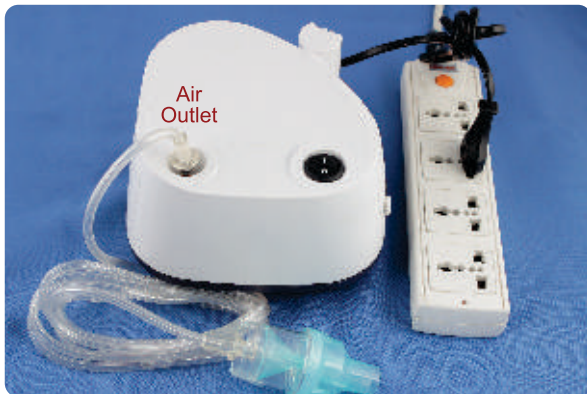
Step 1. Plug-in, connect tube to air outlet
